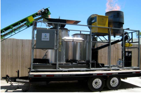
Figure 3. U5 Beta, a mobile continuous flow pyrolysis unit. Photo provided by Biochar Engineering Corp.
