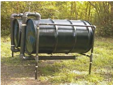
Figure 2. Biochar kiln made from a 55-gallon drum. Photographer unknown.
